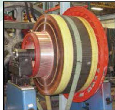
All mechanical repairs on shafts, bearing journals, and end bells, are handled by experienced machinists.
